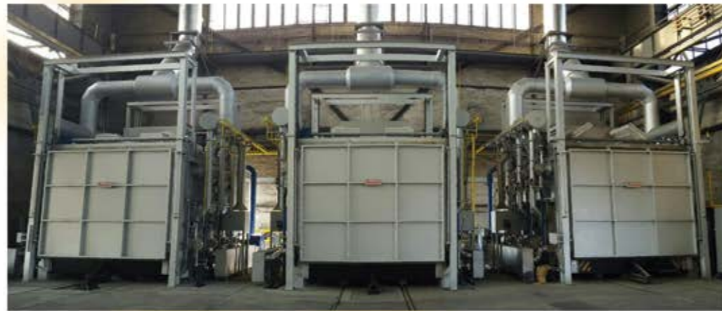
Heat treatment: car-hearth, chamber and shaft furnaces
